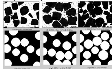
showing simulated architectures adequately capture the thin wall stress concentrations in the struts between pores and pore interconnectivity.
