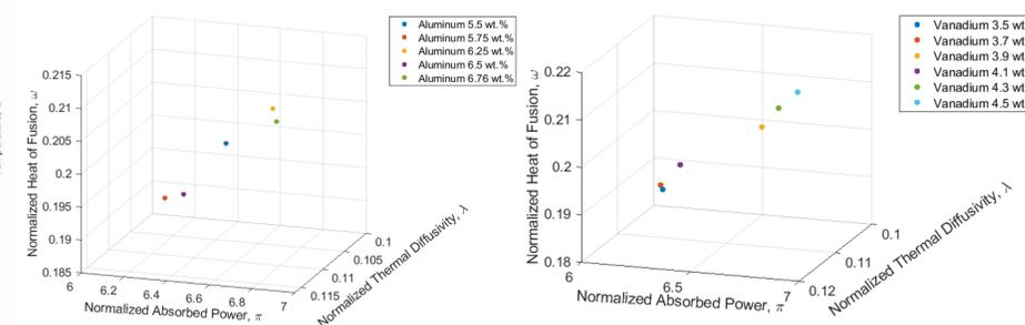
Non-dimensional parameters as a function of aluminum content (left) and as a function of vanadium content (right).
