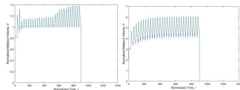
Meltpool volume of different power levels for the reversing lines strategy. Laser power of 60W (left) and laser power of 100 W (right). The meltpool volume throughout the build is qualitatively different.
