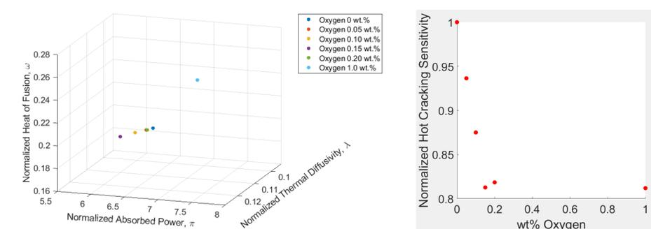
Non-dimensional parameters as a function of oxygen content (left) and a normalized hot cracking sensitivity as a function of oxygen content (right).
