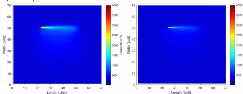
Temperature of top of sector for different power levels for the reversing lines strategy. Laser power of 60W (right) and laser power of 100 W (left). Heat accumulation across the sector is larger at the higher power level.
