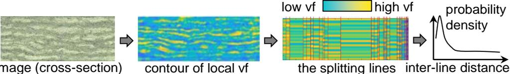
*Modeling:* Regression trees are used to encode the images. Tree nodes are vertical splitting lines and between the lines the vfs are interpolated. Random realizations are generated by sampling from the distribution of the location of the splitting lines.
