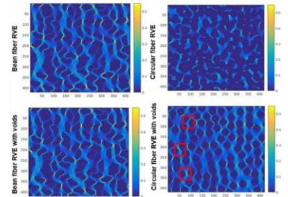
elastic response of RVEs vs experiments using FFT (PBC\* transverse tension)
