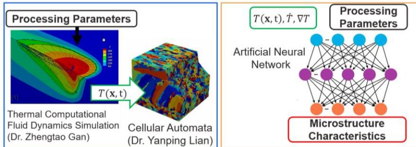
**Neural Networks** Two neural networks were trained on the thermal data to effectively and accurately predict the local average grain size for single-track and multi-track builds. The inputs and outputs of the neural networks are below.
