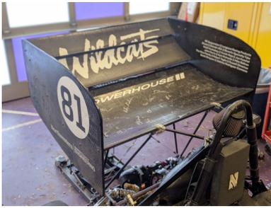
2019 - Carbon Fiber Vehicle Wing Package
