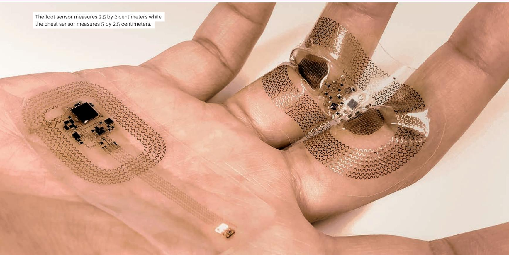
The foot sensor measures 2.5 by 2 centimeters while the chest sensor measures 5 by 2.5 centimeters.
