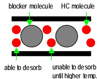
A sketch of a 1-D pore of a zeolite that acts as a “hydrocarbon trap,” which is designed to reduce pollution of conventional gasoline engines.
