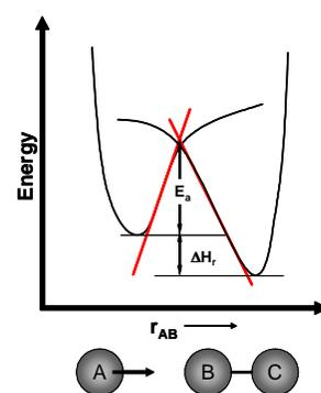
A reaction energy diagram of the reaction  $A + BC \rightarrow AB + C$  illustrates how the Evans-Polanyi relationship relates the activation energy to the reaction enthalpy.
