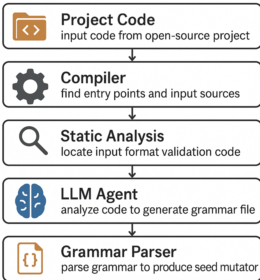
Figure 2.1: Overview of our automated seed-generation framework. Given the source code of an open-source project, the system first analyzes the program through a customized compiler to automatically identify entry points and input sources. It then performs static analysis to locate the code responsible for input parsing and validation, isolating the logic that governs the program’s expected input structure. Building on this extracted information, an LLM-based agent infers a grammar that captures the required format of valid inputs. Finally, the generated grammar is processed by a grammar-based parser, which produces structured seeds that enable the fuzzer to bypass early validation checks and explore deeper program behaviors.
