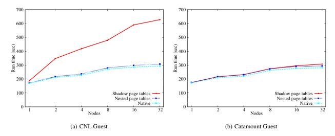
Figure 5: CTH application benchmark comparing scaling for virtualization with shadow paging, virtualization with nested paging, and no virtualization. Palacios/Kitten can provide scaling to 32 nodes with less than 5% performance degradation.
