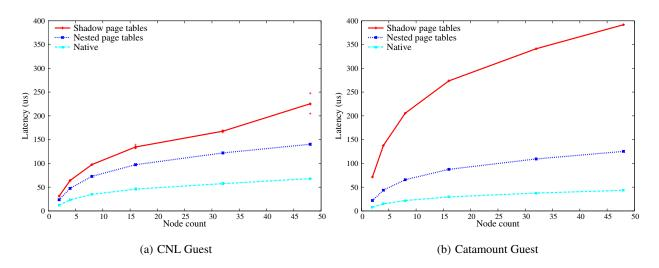
Figure 7: IMB Allreduce 16 byte latency in  $\mu$ sec as a function of nodes up to 48 nodes
