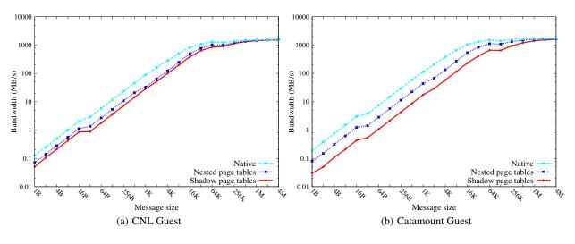
Figure 6: IMB PingPong Bandwidth in MB/sec as a function of message size
