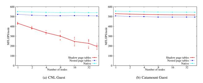
Figure 4: HPCCG benchmark comparing scaling for virtualization with shadow paging, virtualization with nested paging, and no virtualization. Palacios/Kitten can provide scaling to 48 nodes with less than 5% performance degradation.
