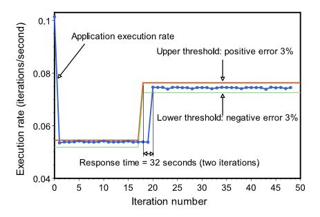
Figure 6.6: Response time of control algorithm; 1:1 comp/comm ratio.
