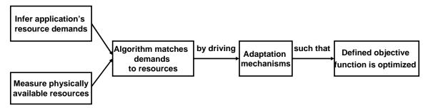
Figure 1.1: The core of a generic adaptive system.
