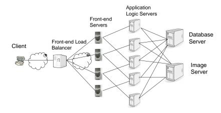
Figure 2.5: A schematic model of an enterprise database application.
