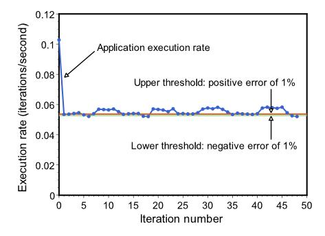
Figure 6.5: System in oscillation when error threshold is made too small; 1:1 comp/comm ratio.
