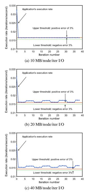
Figure 6.13: Performance of control system with a high (145:1) comp/comm ratio and varying local disk I/O.
