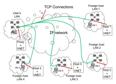
Figure 3.12: VNET startup topology.
