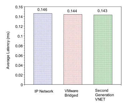
Figure 3.17: Average latency over a 100 Mbit switch with different bottlenecks.
