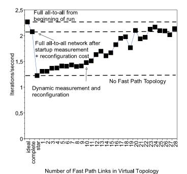
Figure 8.5: All-to-all topology with eight VMs, spread over a WAN.
