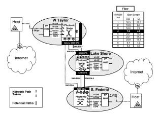
Figure 5.1: Physical topology of the OMNInet testbed network.
