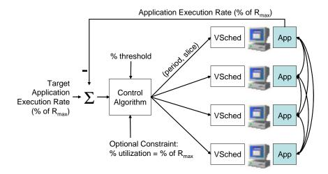
Figure 6.1: Structure of global control.
