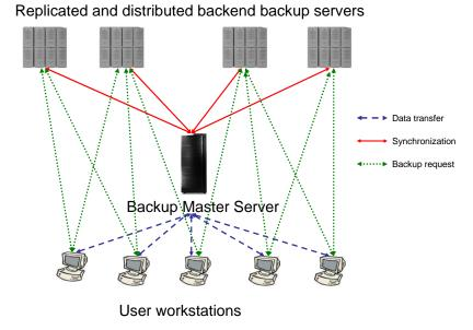
Figure 2.2: A schematic model of enterprise backup applications.
