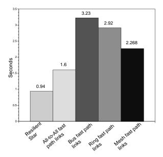
Figure 8.1: Time to set up the backbone star configuration and to add fast path links for different (inferred) topologies.
