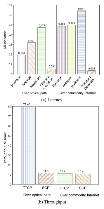
Figure 5.3: Latency and throughput of the optical path as compared to the commodity Internet.
