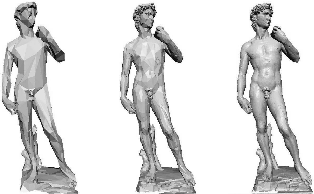
Figure 6: David model (28 million vertices) simplified to roughly 1000 vertices (left), 5000 vertices (middle) and 50,000 vertices (right), using VMRSimp (bottom) and adaptive simplification (top). Note the extraneous joints at the groin and armpits in adaptive simplification. Again, the flipped normals in adaptive simplification could easily be fixed.
