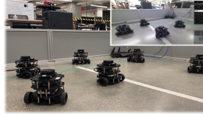
Figure 3.1. This figure shows DOS® deploy a collision-free navigation algorithm to a swarm of robots. (Turtlebot Burger). The right-top figure is the Operating page where viewing from the coach robot (Pyrobot). User can manually move the robot by the joystick the page provides.
