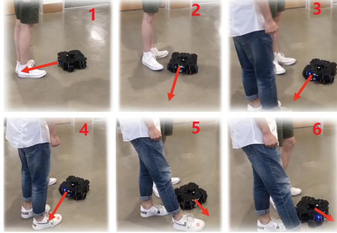
Figure 3.8. A real-world deployment. We deploy our collision avoidance policy on turtlebot3. The red arrows represent the moving directions of the robot. The result shows that when two pedestrians try to maliciously block the robot, our trained collision avoidance policy still find a collision-free path for the robot.
