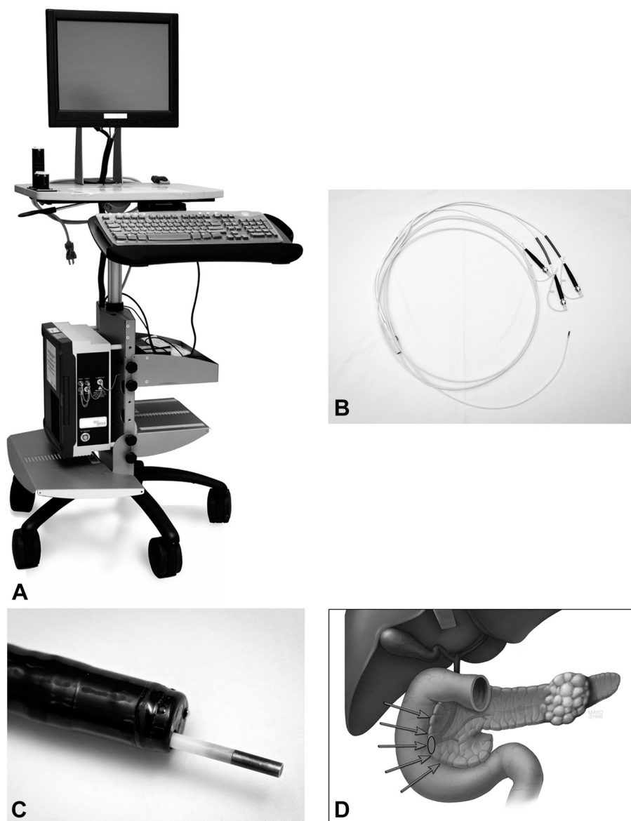
Figure 2. A , Spectroscopy processor, monitor, and keyboard of PGS measurement unit. B , Fiberoptic probe of polarization gating spectroscopic measurement unit. C , Polarization gating fiberoptic probe fed through the accessory channel of the standard upper endoscope. D , Periampullary locations where spectroscopy measurements were obtained.
