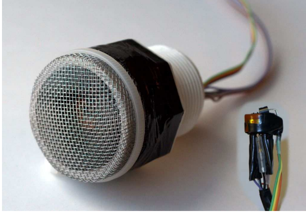
Figure 12: Insulated carbon monoxide sensor assembly, with metal screen to diffuse the wind. Inset shows the internal structure of the sensor; a temperature sensor is on top of the MQ-7 carbon monoxide sensor, and the resistor that serves as a supplementary heater is attached to the bottom of the MQ-7 sensor.
