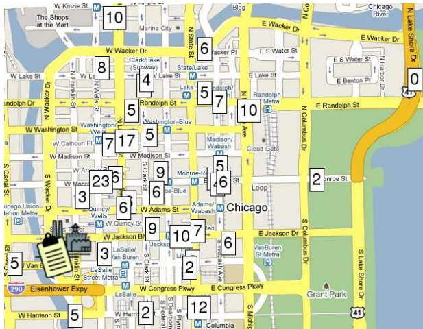
Figure 13: Map of measured CO concentration (ppm) in downtown Chicago. Each value is centered on the position at which the measurement was taken. All data points were collected within two hours. The icon of a building in the lower left corner represents the only stationary monitoring node in the Illinois air monitoring network in downtown Chicago; the next closest station is 10 km away.
